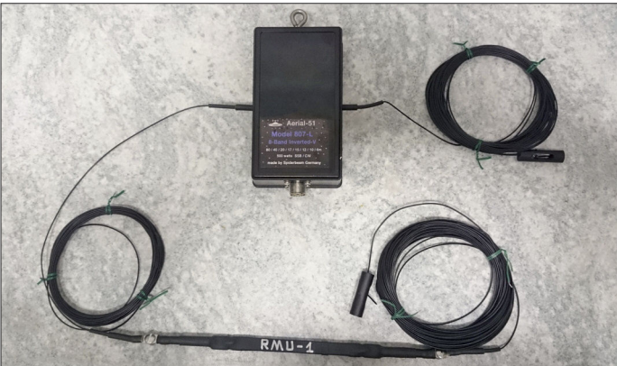
Fig. 1. This handy sized bundle of a hybrid balun (above), a long wire leg including an RMU Remote Matching Unit (below), and a short wire leg (top right) fits into a large pants pocket.
