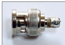
Figure 89: BNC connector with folded and shortened wire
