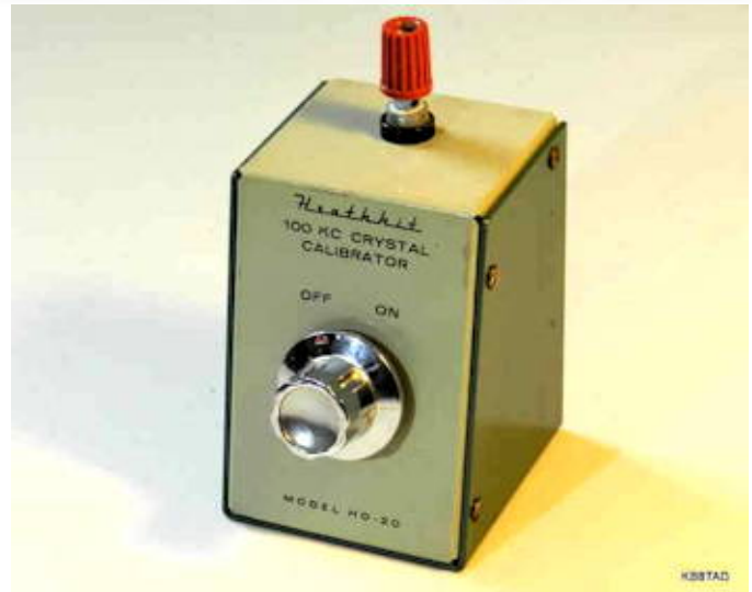
Figure 1: Heathkit HD-20 100 kc Crystal Calibrator. Photo courtesy of Richard Post - KB8TAD
