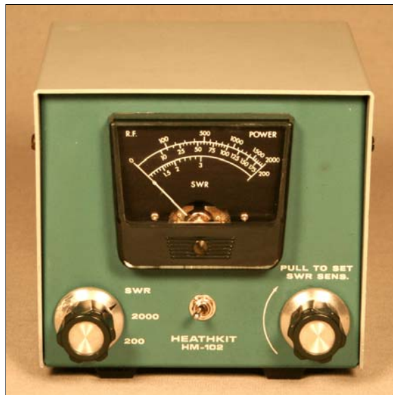
Figure 2 - Reconditioned HM-102 with Added Forward/Reflected Toggle Switch
