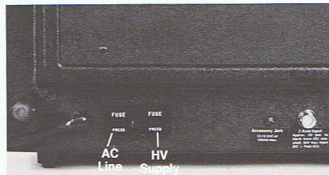
Fig. 43 — Location of the fuses and jacks on the back panel.
