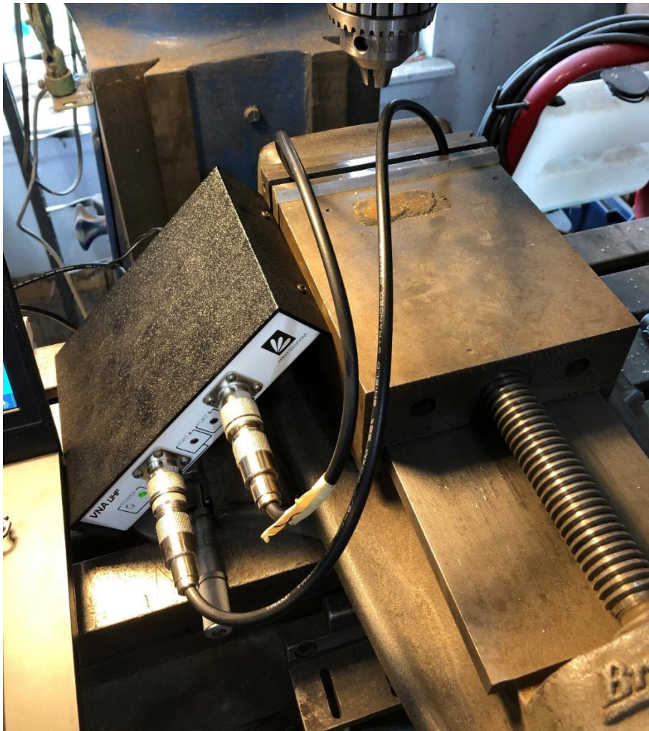
Figure 11: Smash test was done in a milling machine vise because the jaws are absolutely flat, absolutely parallel, coplanar, and it's very easy to measure compression with an ID micrometer.
