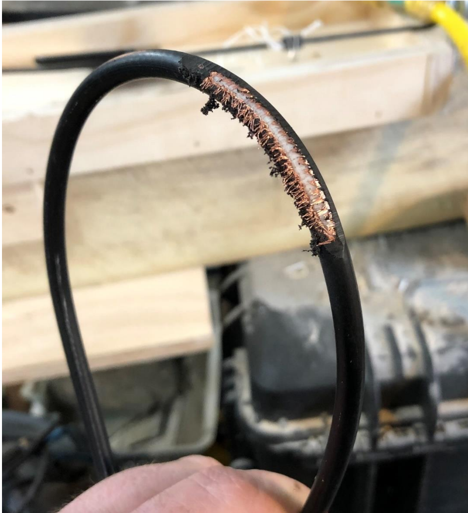
Figure 18: Bench grinder to simulate perhaps a little abrasion. "[we dragged it] over the hills and through the woods to grandma's house!"
