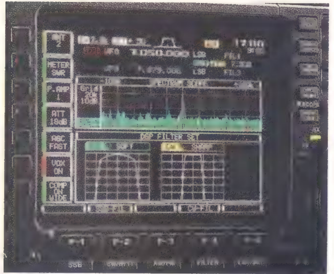
Photo 3: The large LCD screen displaying the mini spectrum scope and the filters. Note the graphical representations of the 'soft' and 'sharp' filter shapes.
