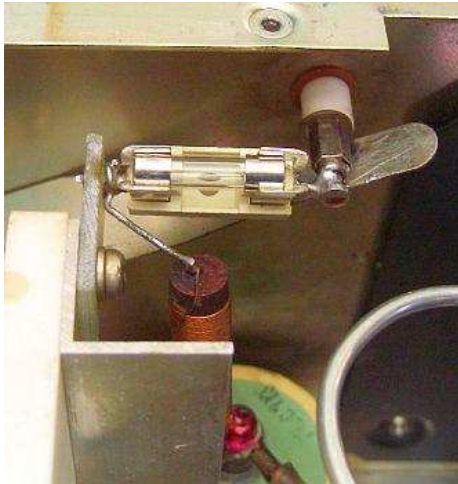
Mounting in another TL-922. The resistor was glued with Cyanoacrilate.
