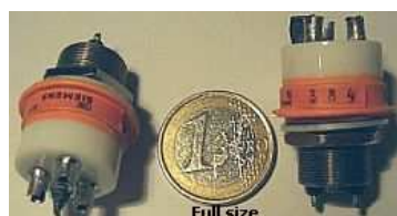
Relay1 SIEMENS vacuum relay VR311, 26.5 V/335 Ω, suited for 8 kV/8 A at 30 MHz
