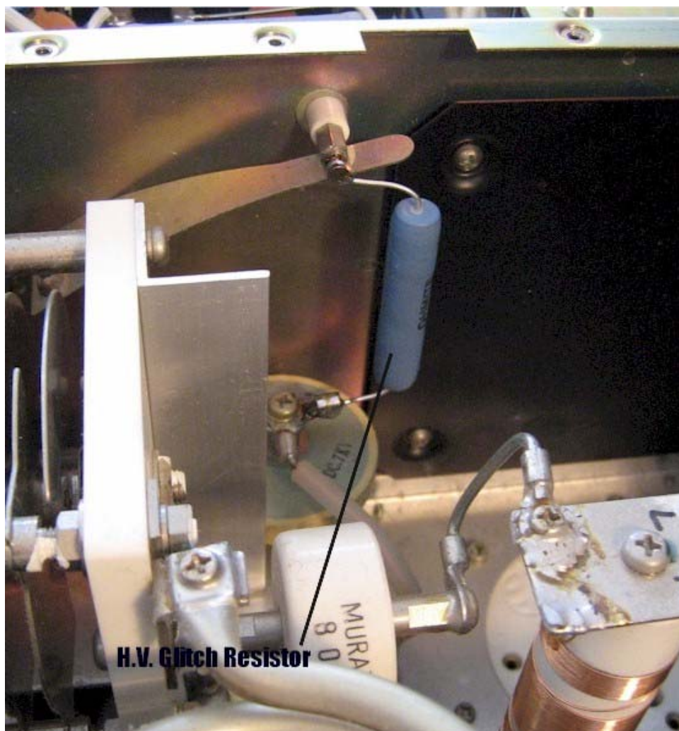
Original inductor L2 replaced with a 10 ohm 'glitch' protection resistor in high voltage supply.
