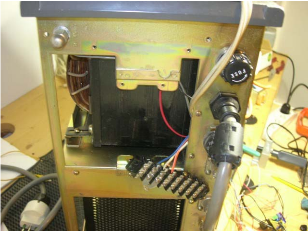
Fig. 20 – Removal of the band switch
