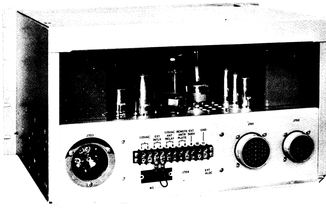
Figure 1-2b. Rear Angle View, PS-4A Low Voltage Power Supply
