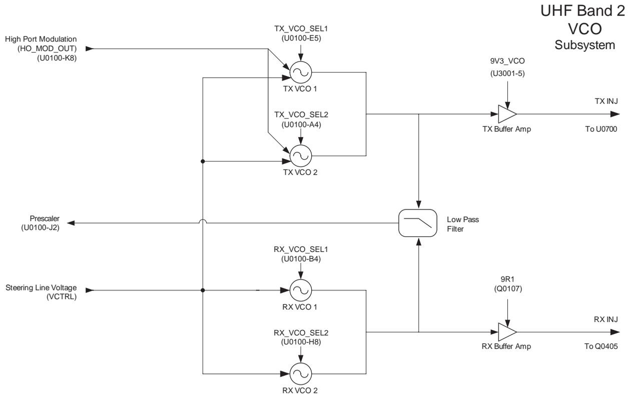
Figure 1-10 UHF Band 2 VCO Block Diagram
