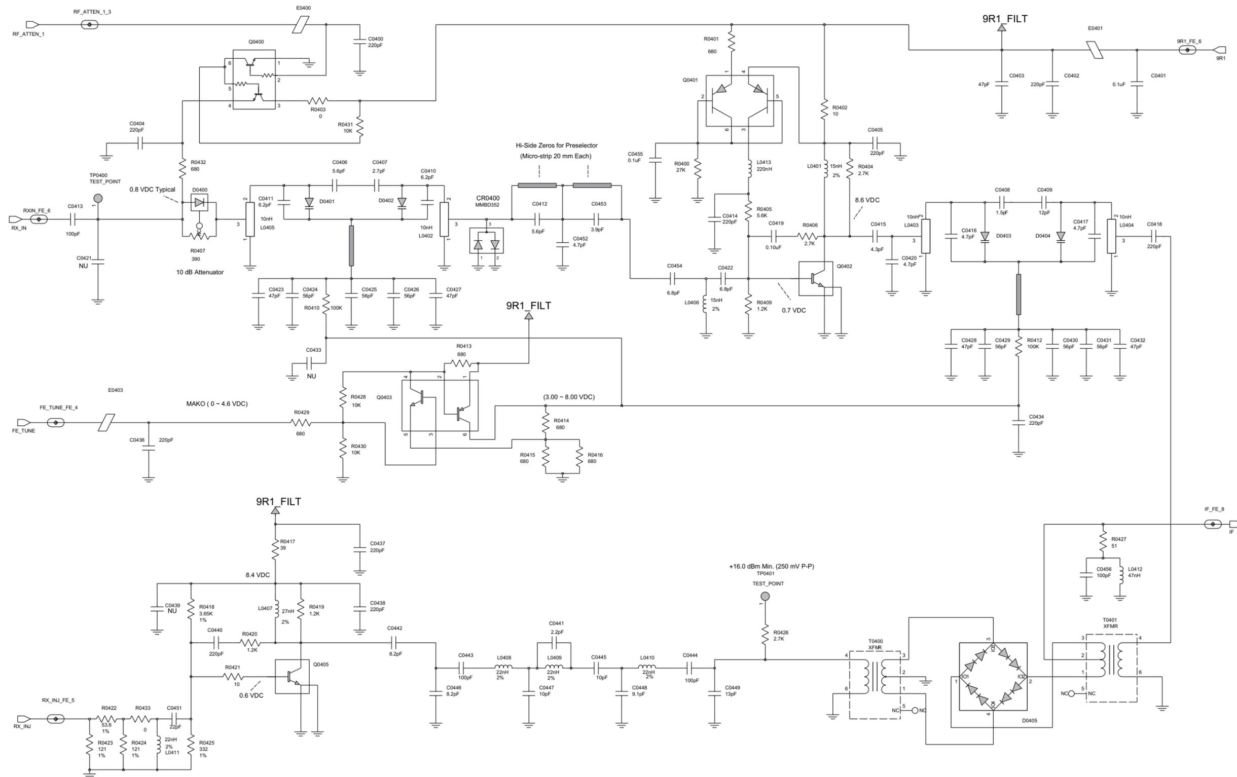
UHF1 (403-470 MHz) 1-25W Receiver Front-End Schematic Diagram
