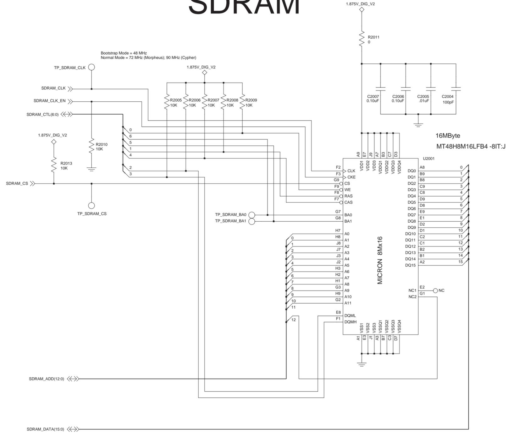
Controller Memories Schematic Diagram
