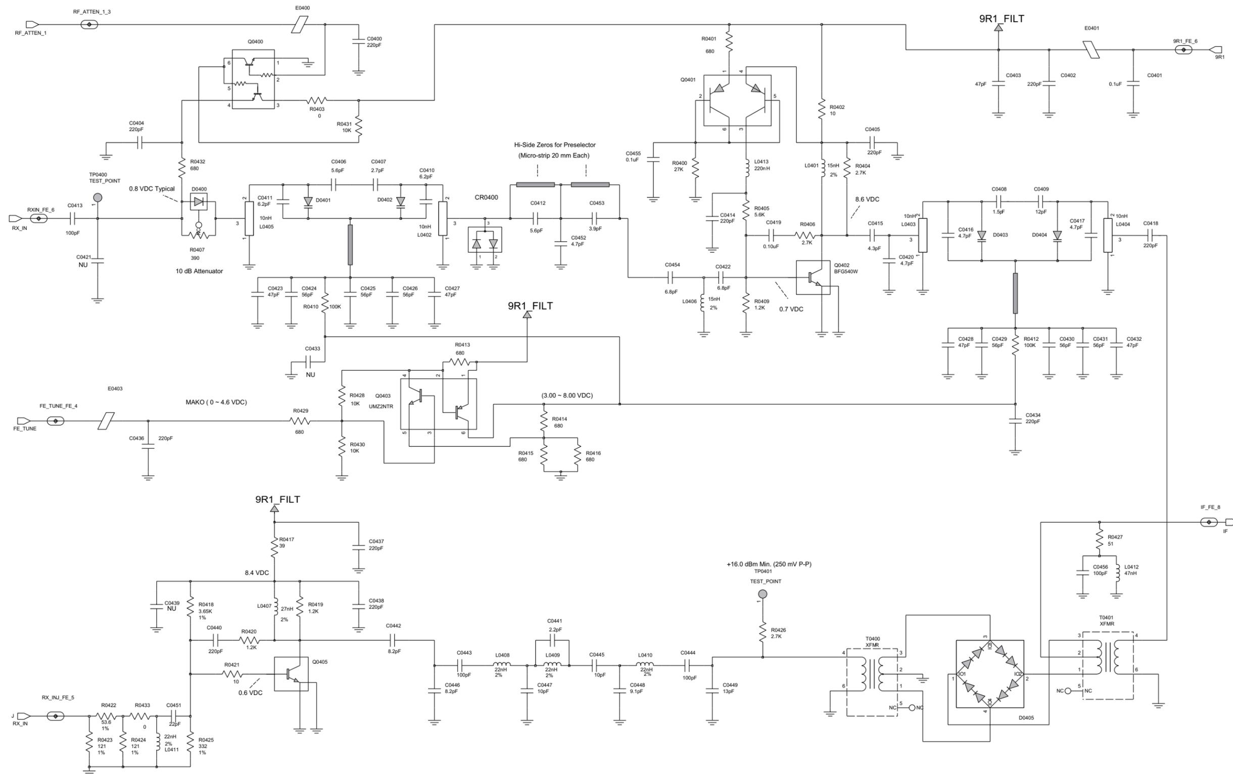
UHF1 (403-470 MHz) 25-40W Receiver Front-End Schematic Diagram
