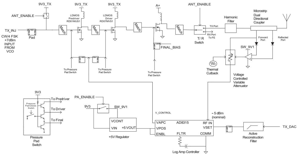
Figure 1-8 VHF 25 Watt Low-Power Transmitter Detailed Block Diagram
