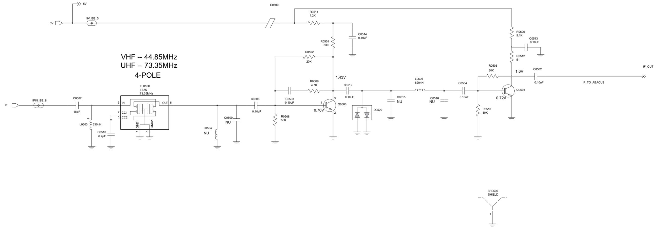
UHF1 (403–470 MHz) 25–40W Receiver IF Amp Schematic Diagram
