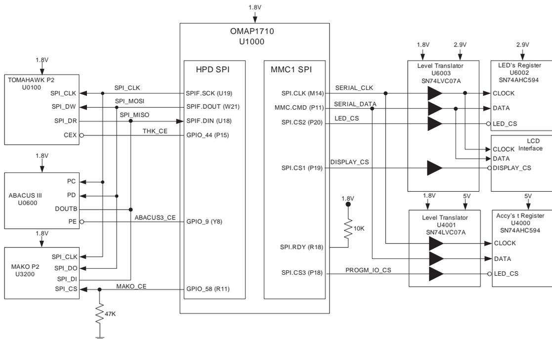
Figure 1-5 SPI Connections
