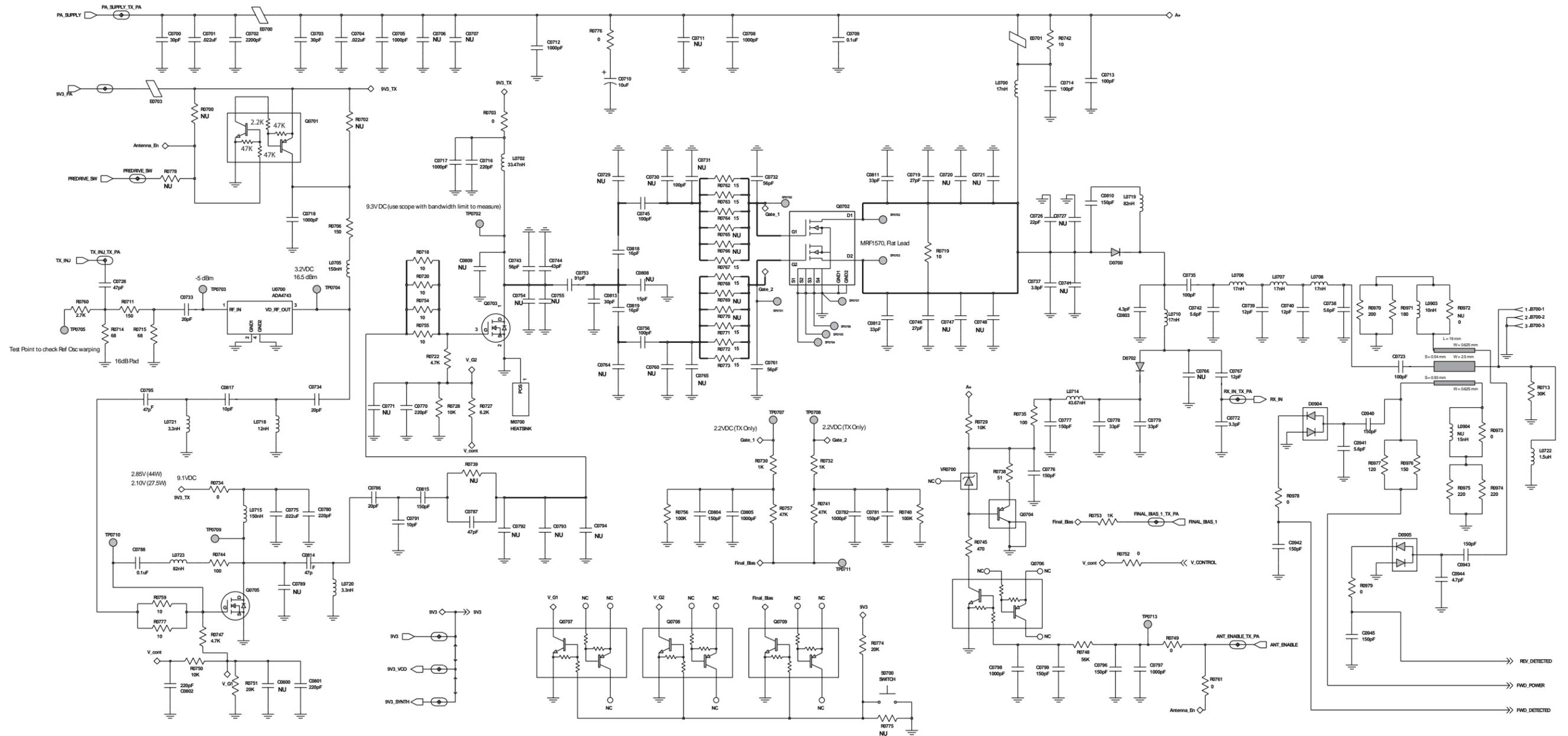
UHF1 (403–470 MHz) 1–25W Power Amplifier Schematic Diagram
