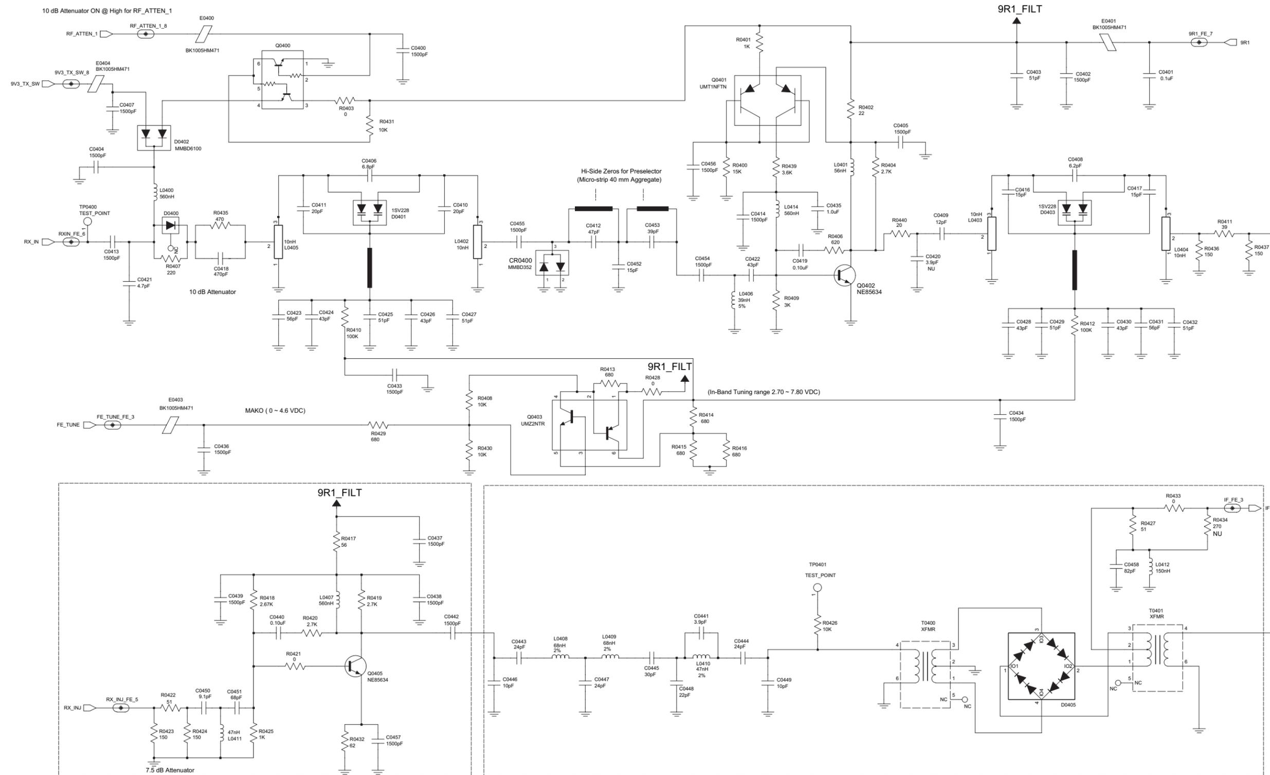
VHF (136-174 MHz) 1-25W Receiver Front-End Schematic Diagram
