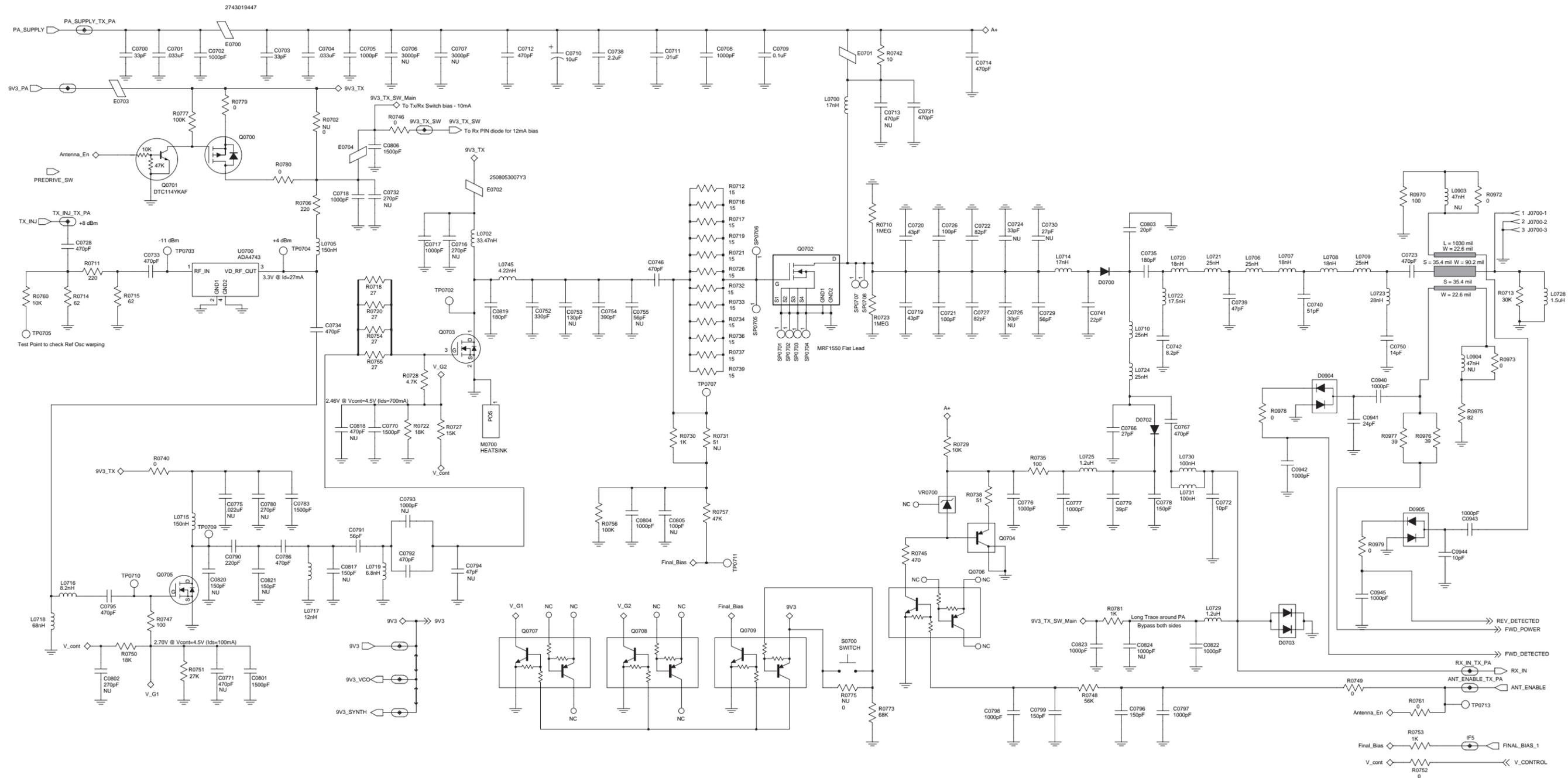
VHF (136–174 MHz) 25–45W Power Amplifier Schematic Diagram
