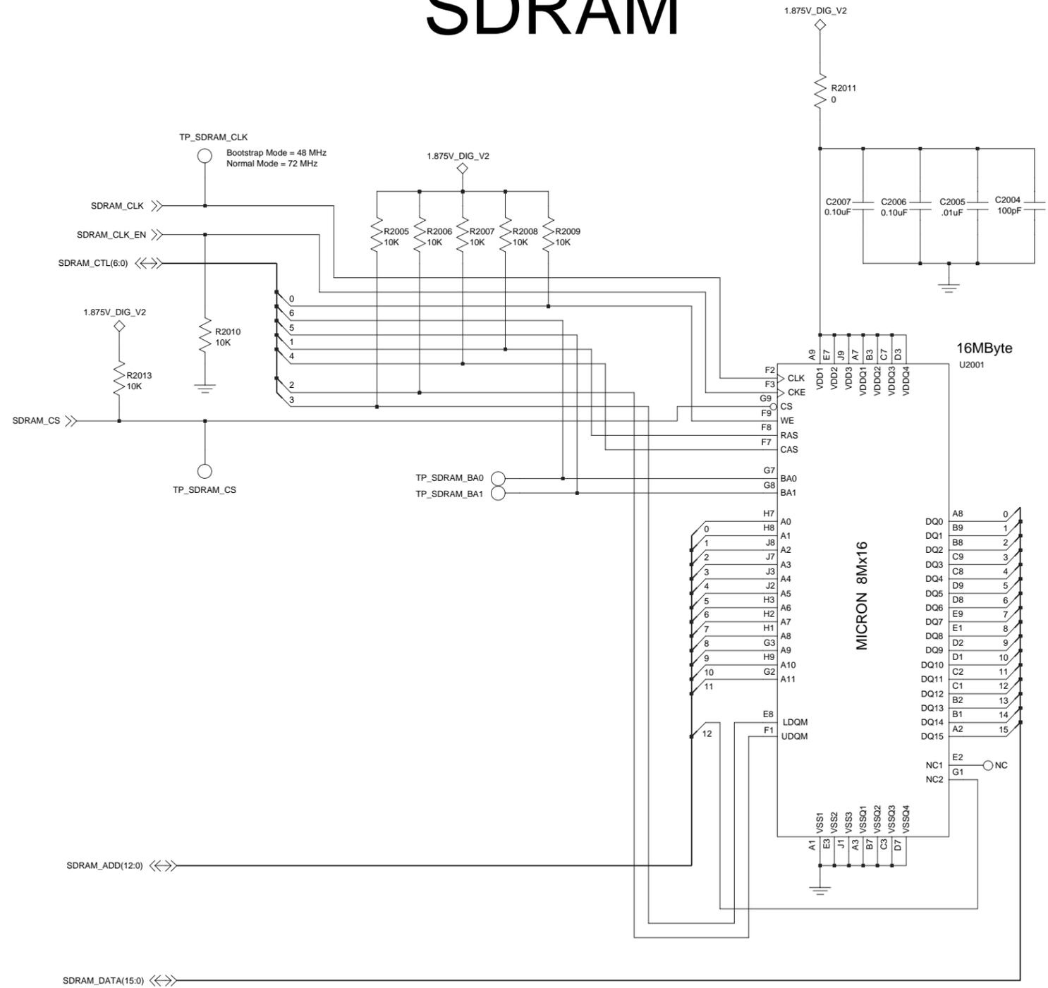
Controller Memories Schematic Diagram
