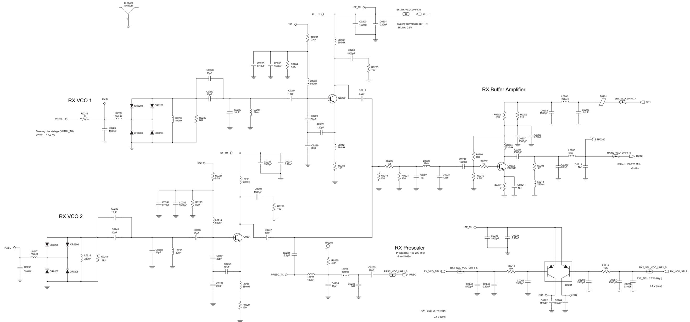
VHF (136–174 MHz) 1–25W Receiver VCO Schematic Diagram
