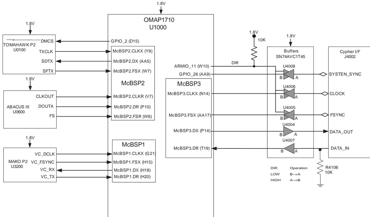
Figure 1-6 SSI Connections
