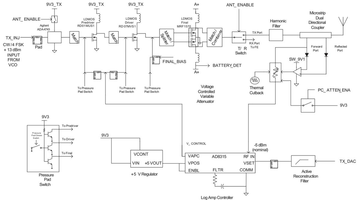
Figure 1-8 UHF 25 Watt Low-Power Transmitter Detailed Block Diagram
