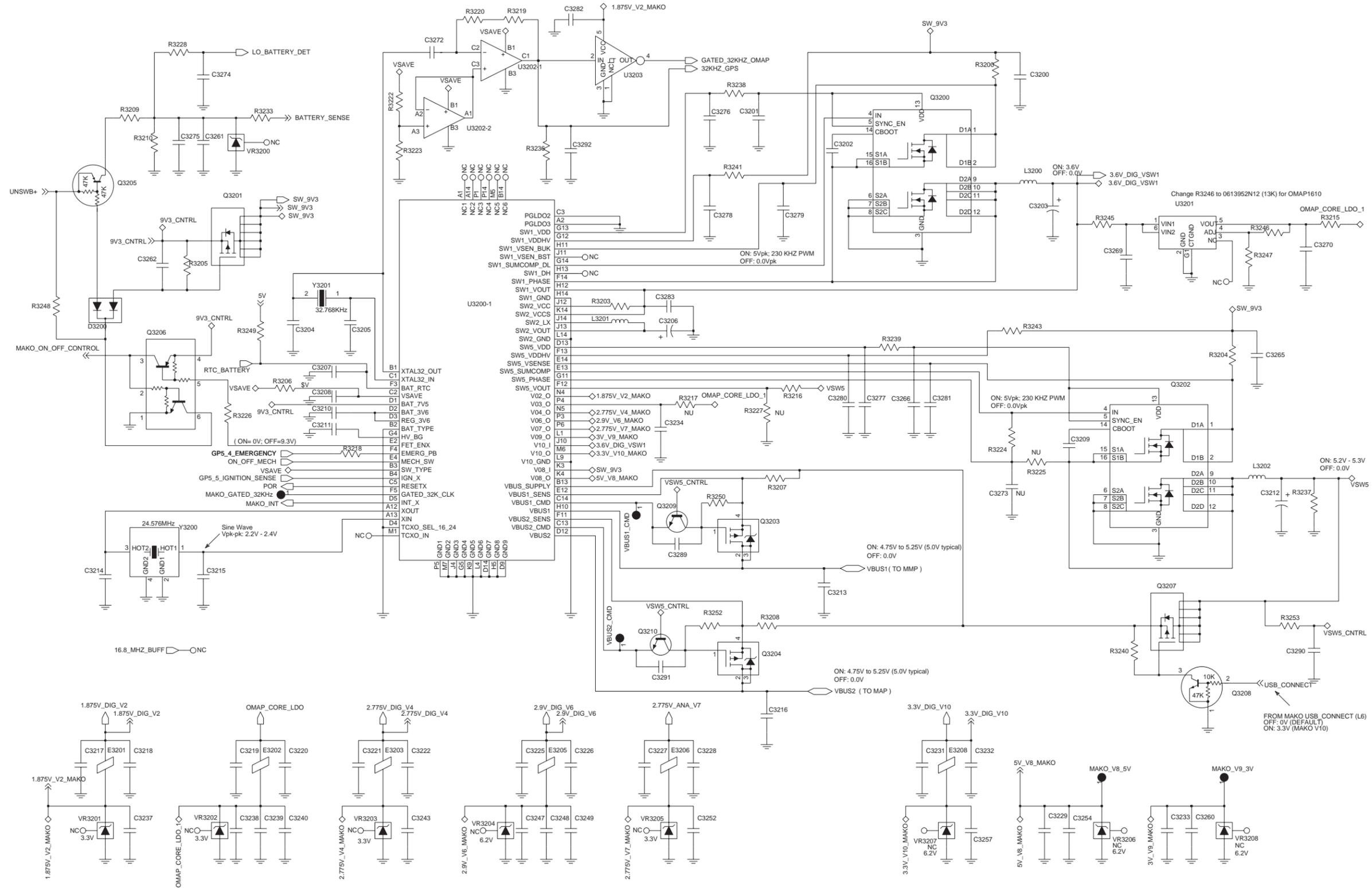
Controller DC Distribution Schematic Diagram
