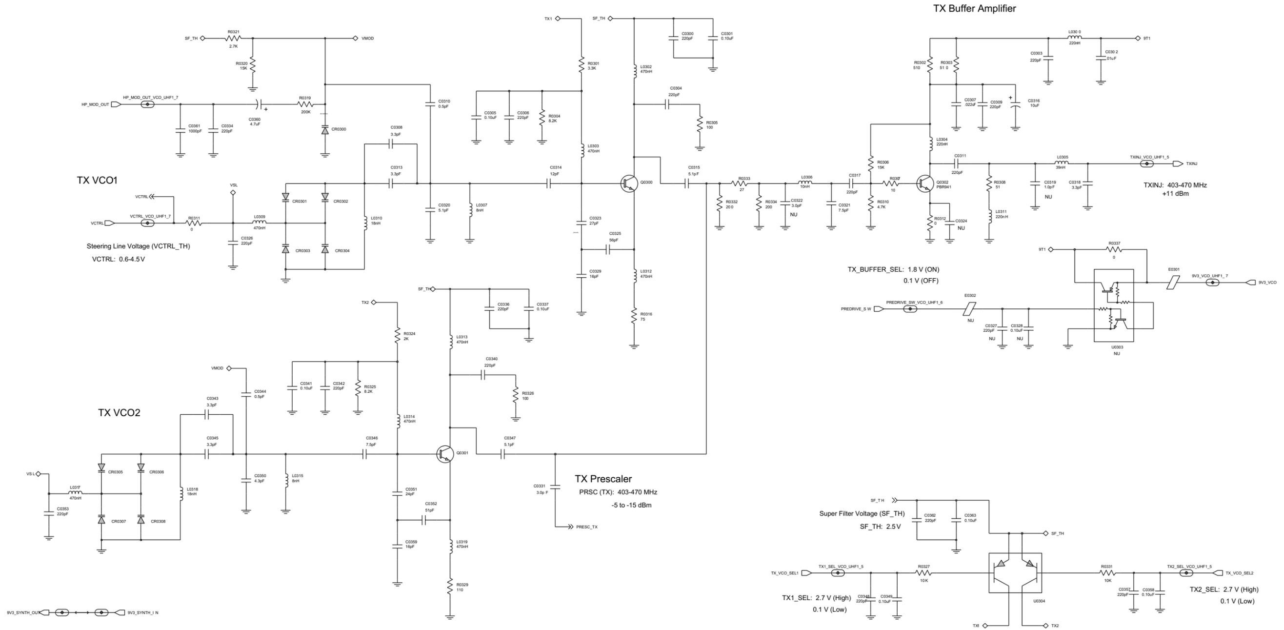
UHF1 (403-470 MHz) 25-40W Transmit VCO Schematic Diagram
