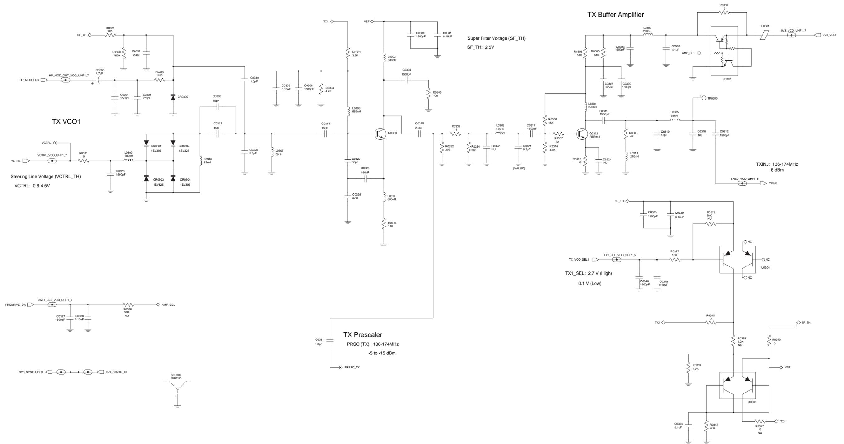
VHF (136-174 MHz) 25-45W Transmit VCO Schematic Diagram
