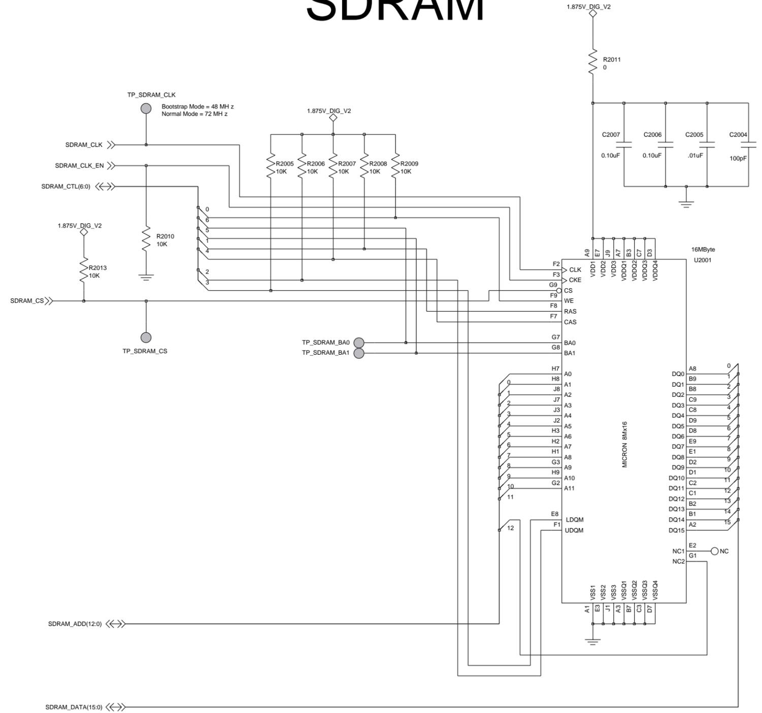
Controller Memories Schematic Diagram
