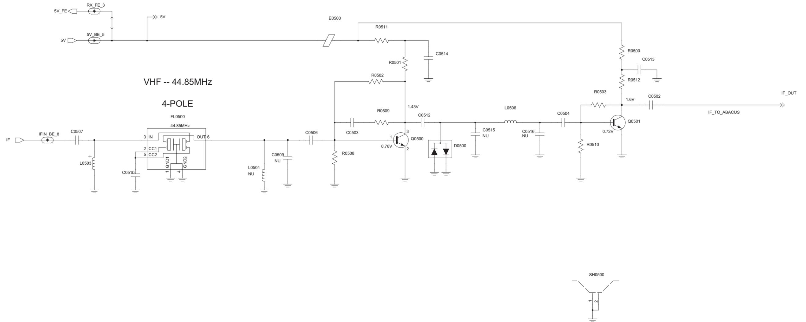
VHF (136–174 MHz) 1–25W Receiver IF Amp Schematic Diagram
