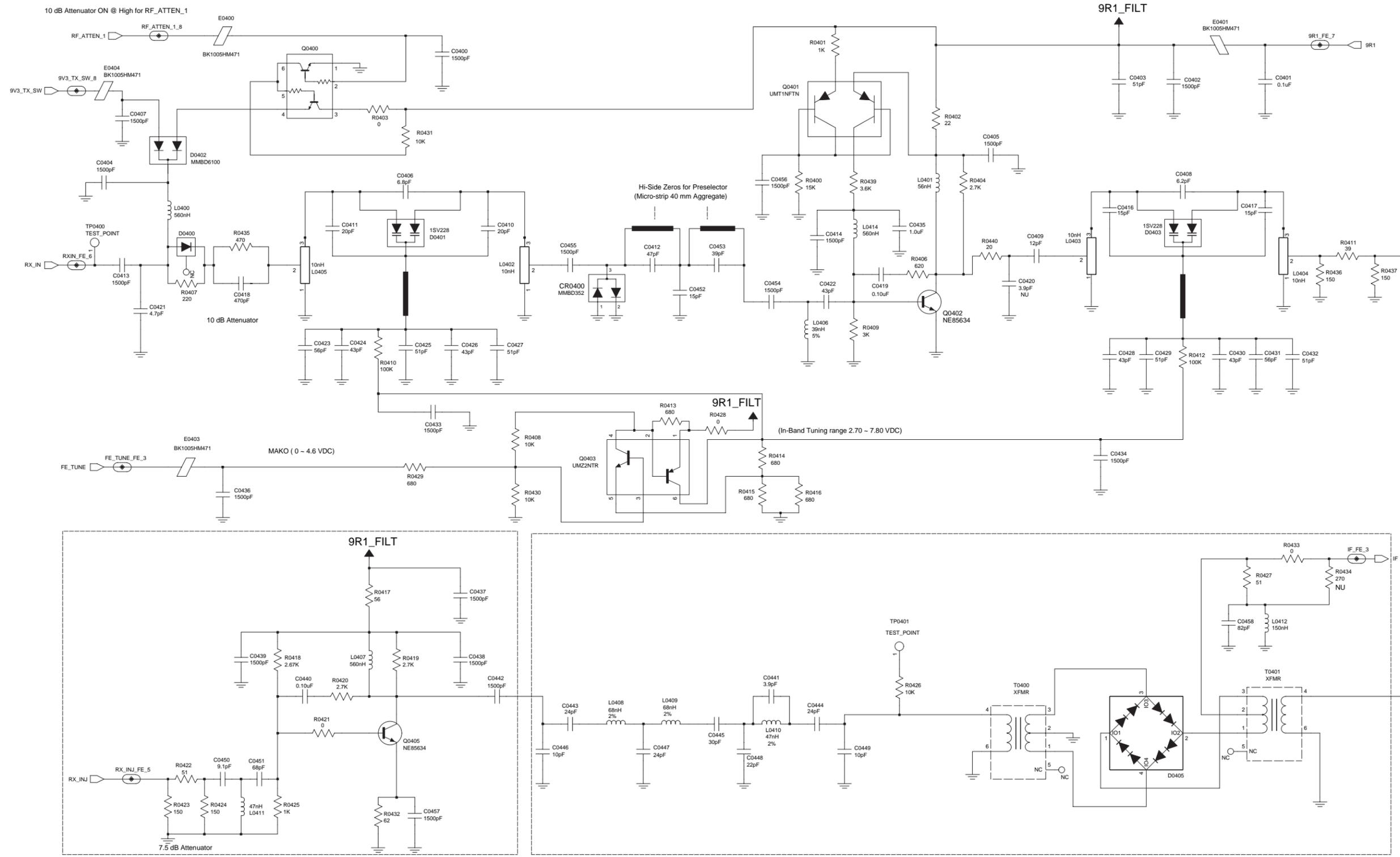
VHF (136-174 MHz) 25-45W Receiver Front-End Schematic Diagram
