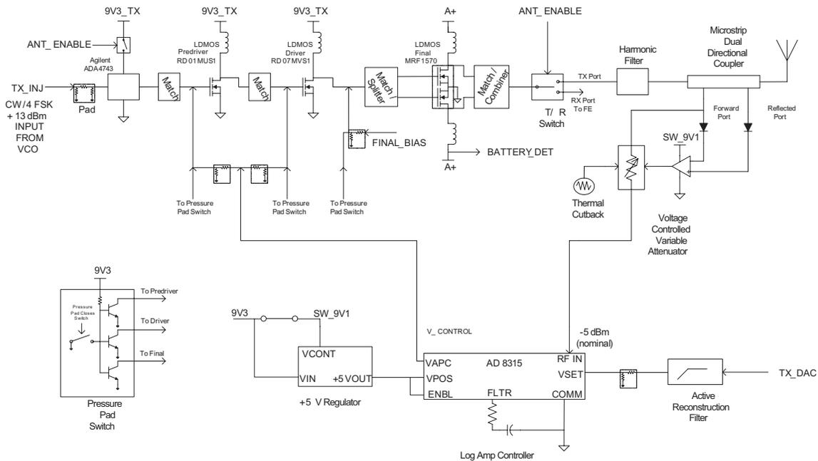
Figure 1-8 UHF 40 Watt High-Power Transmitter Detailed Block Diagram
