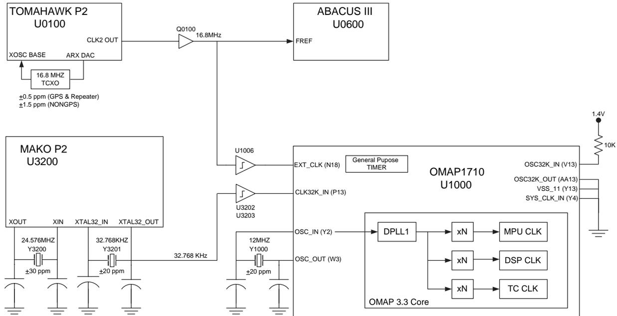
Figure 1-4 Clock Connections
