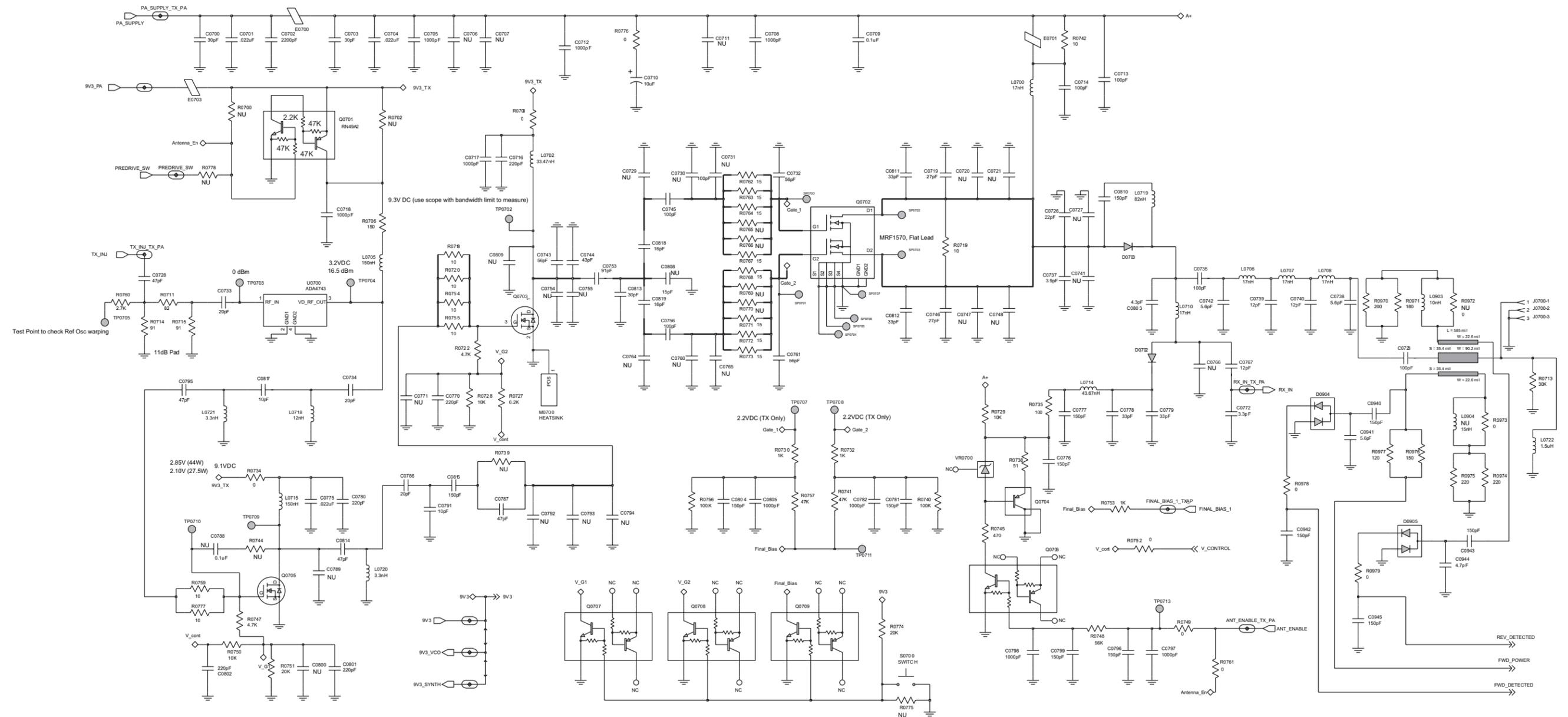
UHF1 (403–470 MHz) 25–40W Power Amplifier Schematic Diagram
