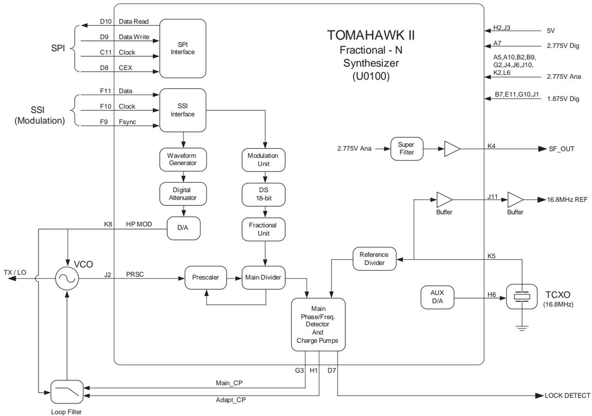
Figure 1-9 UHF Band 2 Synthesizer Block Diagram
