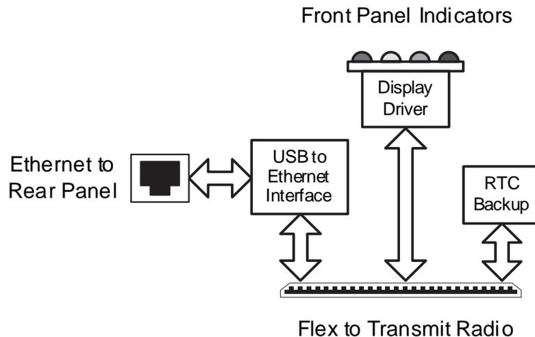
*Figure 1-1 Repeater Indicator Board Block Diagram*
