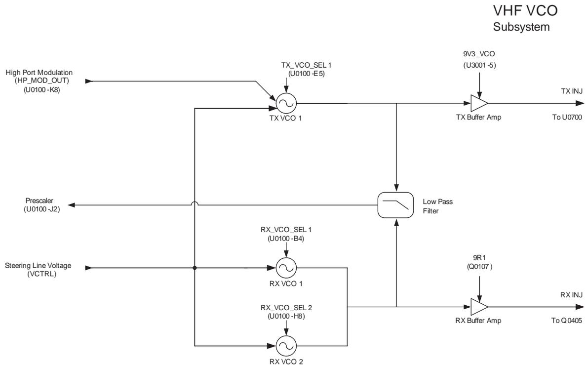
Figure 1-10 VHF VCO Block Diagram
