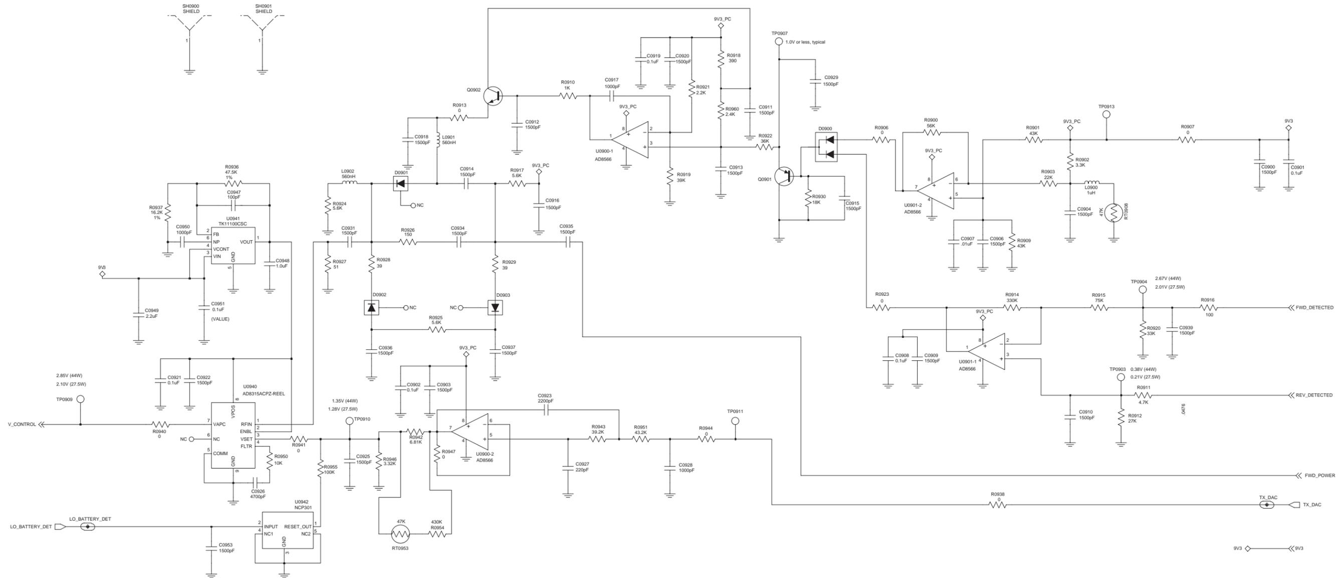
VHF (136-174 MHz) 25-45W Power Control Schematic Diagram
