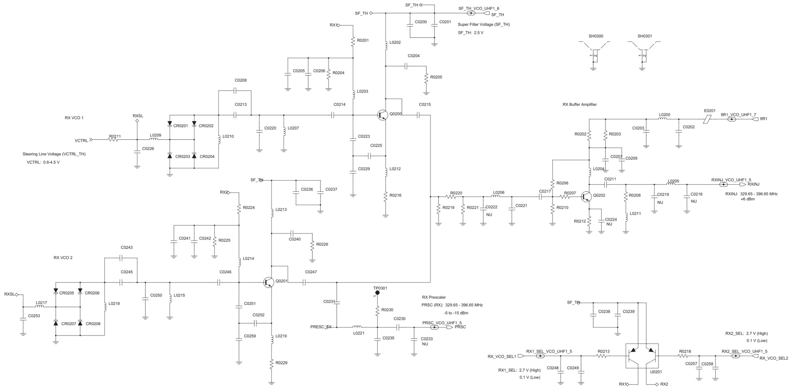
**UHF1 (403–470 MHz) 1–25W Receiver VCO Schematic Diagram**
