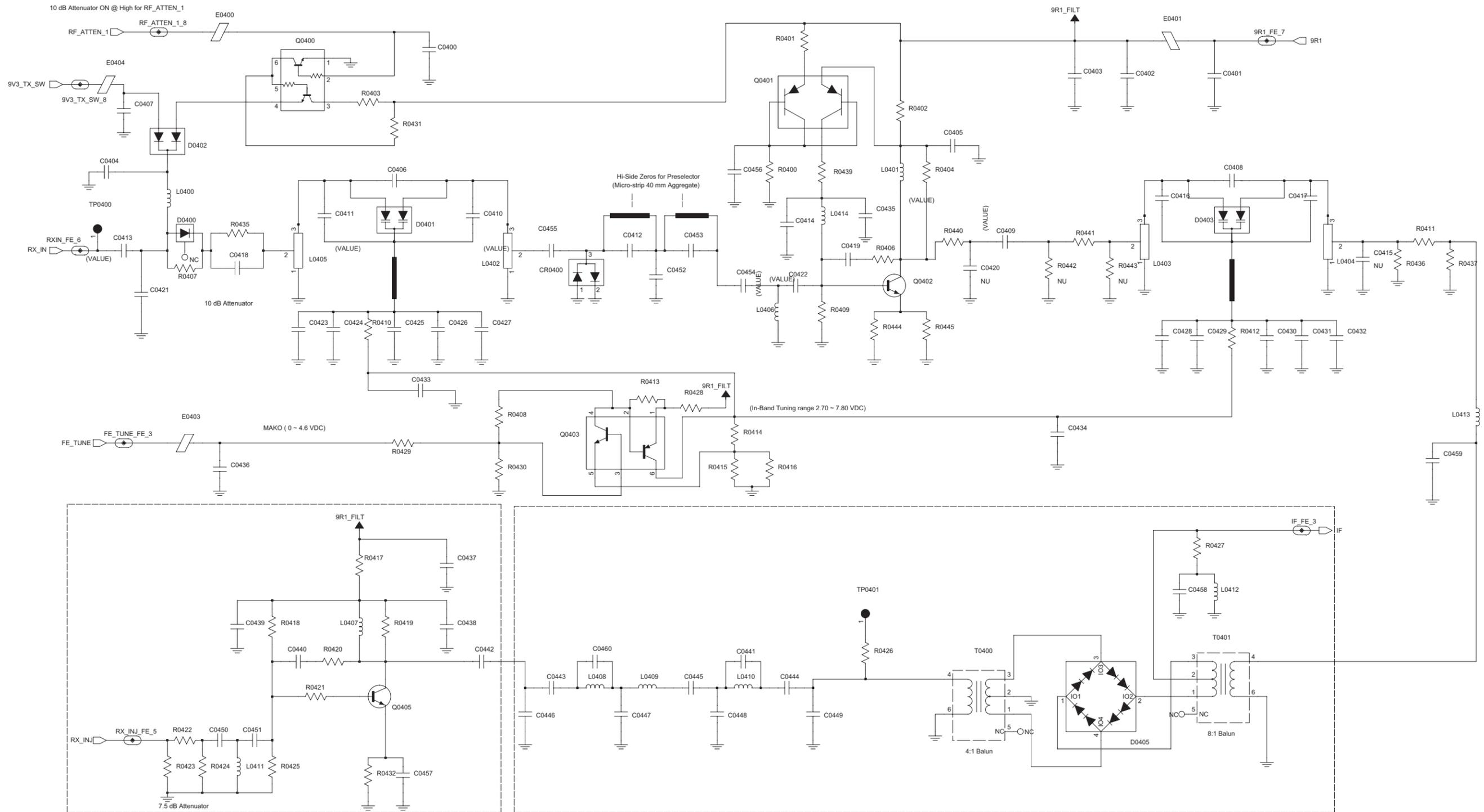
VHF (136-174 MHz) 1-25W Receiver Front-End Schematic Diagram
