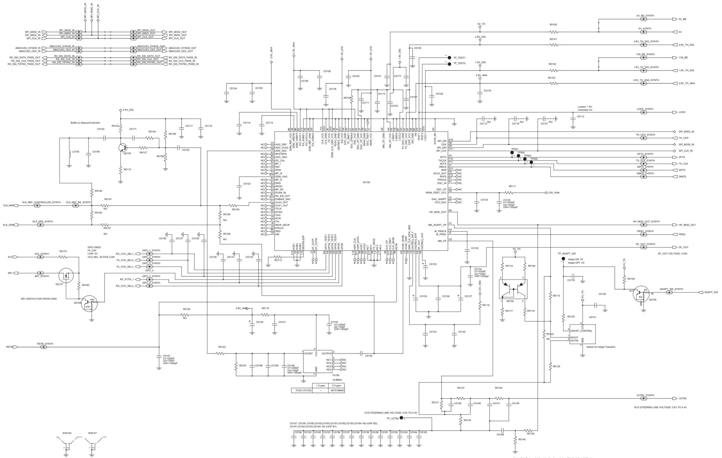
UHF1 (403–470 MHz) 25–40W Synthesizer Schematic Diagram
