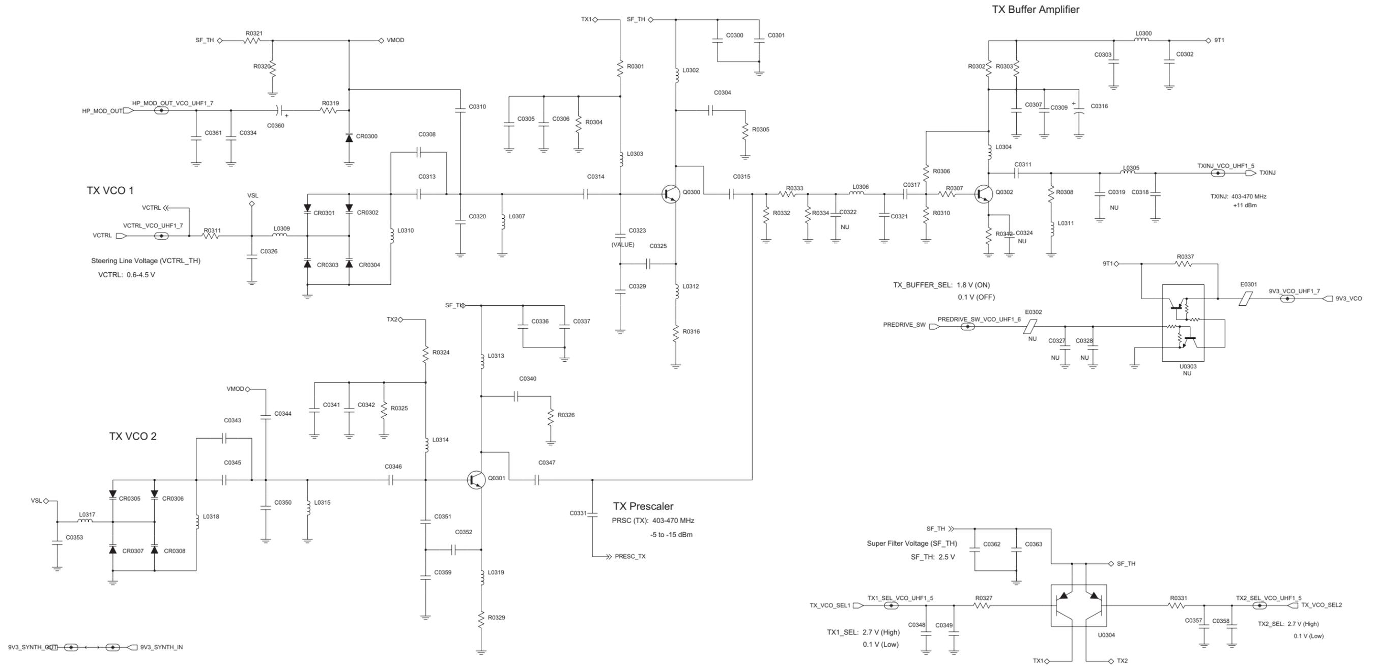
**UHF1 (403-470 MHz) 25-40W Transmit VCO Schematic Diagram**
