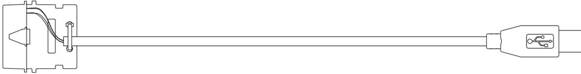
Figure 3-1 Mobile & Repeater Rear Programming Cable PMKN4010\_
