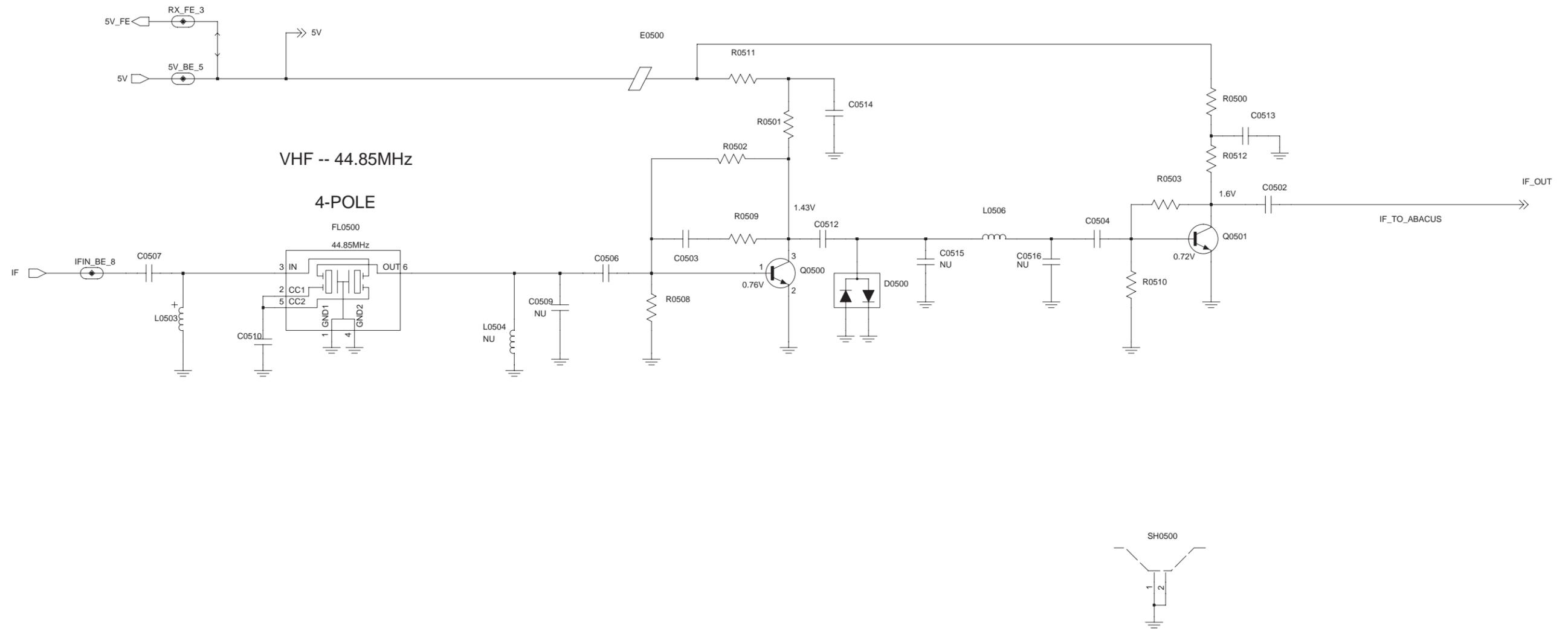
VHF (136–174 MHz) 25–45W Receiver IF Amp Schematic Diagram
