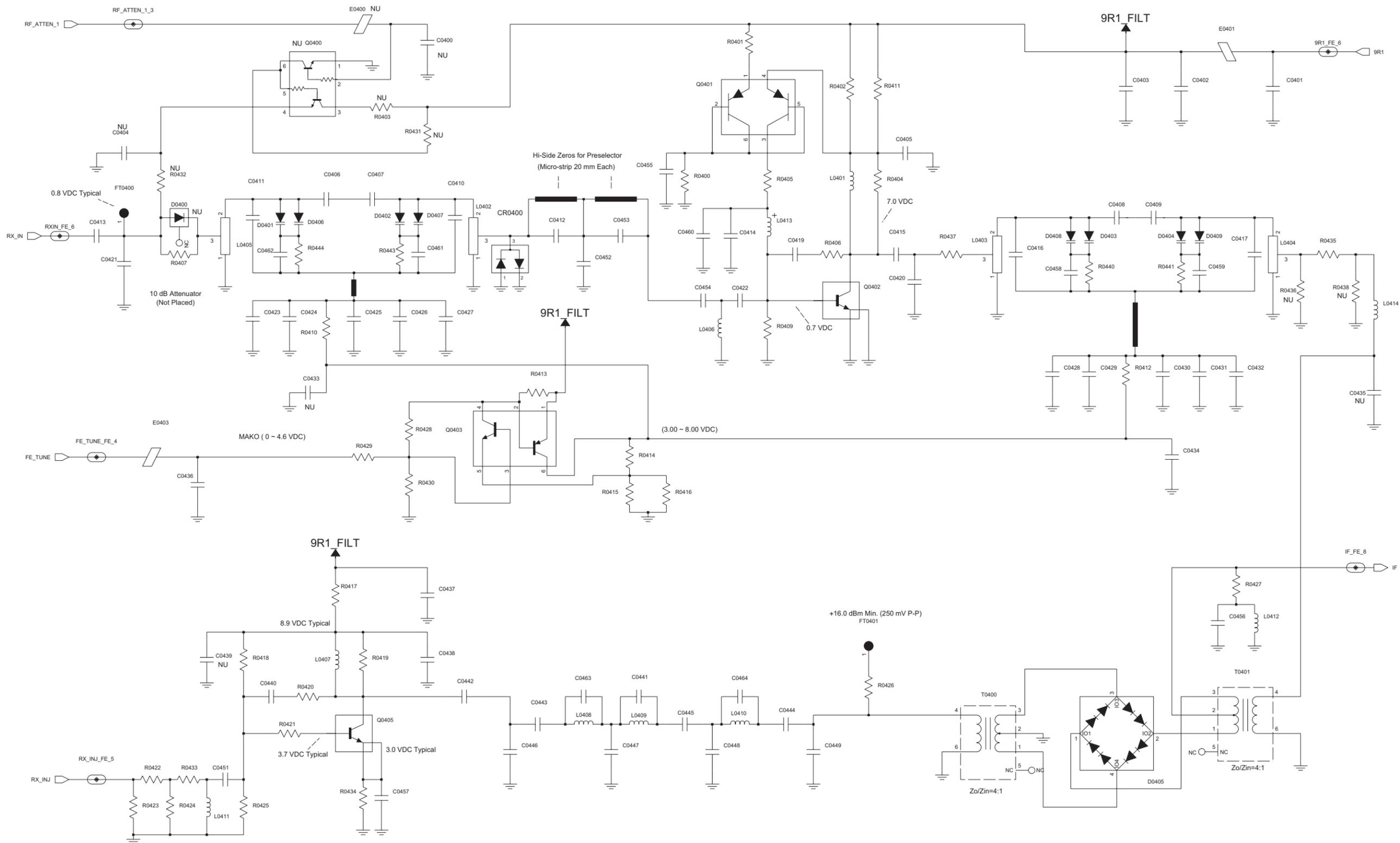
UHF1 (403-470 MHz) 25-40W Receiver Front-End Schematic Diagram
