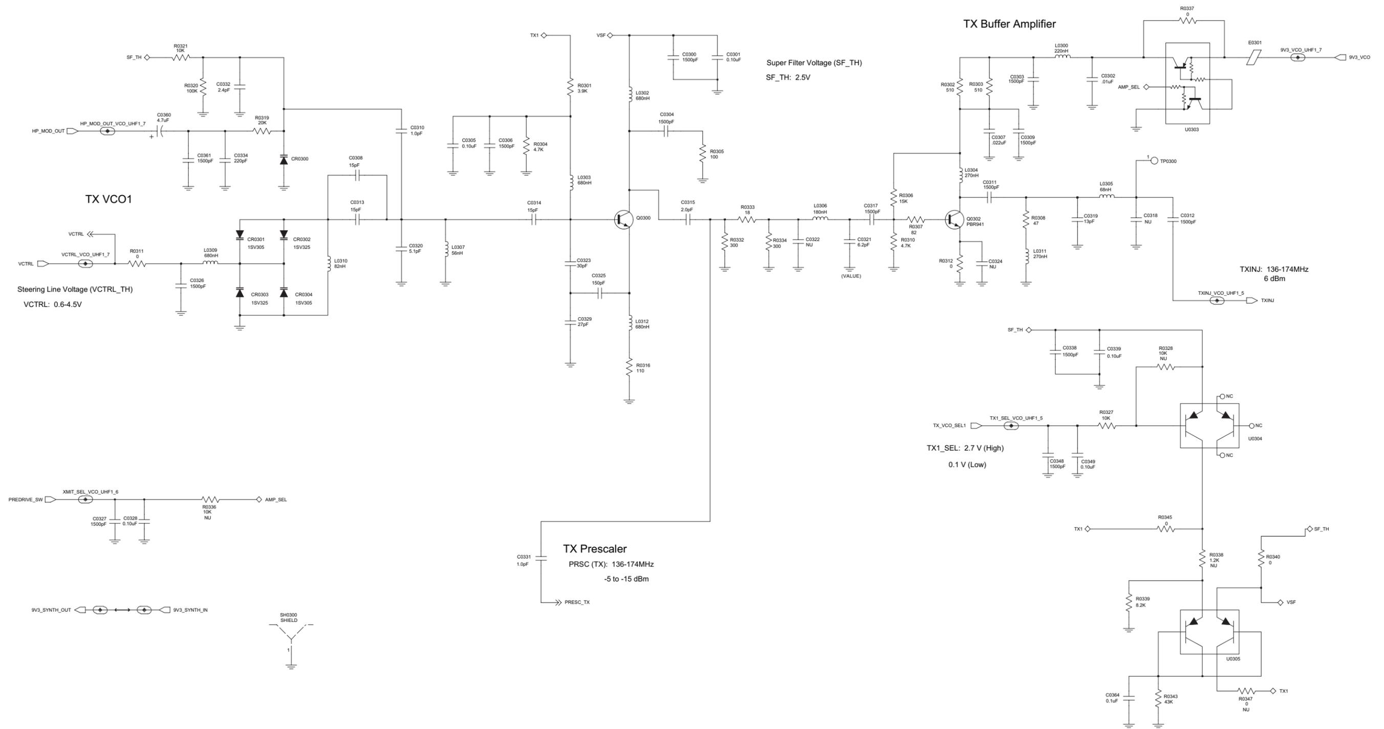
VHF (136–174 MHz) 1–25W Transmit VCO Schematic Diagram
