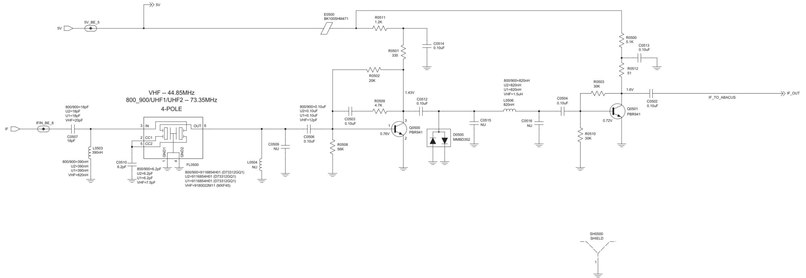
UHF2 (450–527 MHz) 1–40W Receiver IF Amp Schematic Diagram
