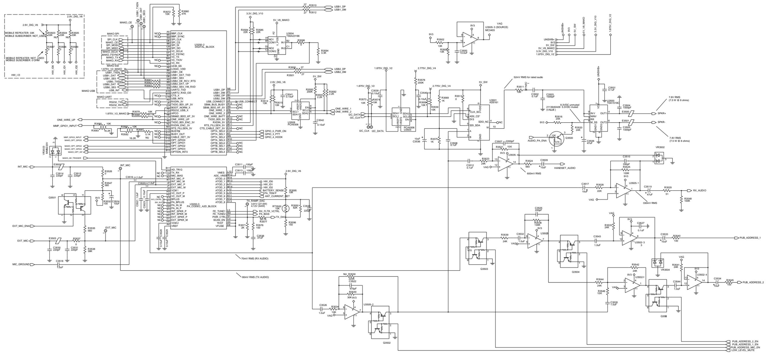
Controller Audio and USB Schematic Diagram
