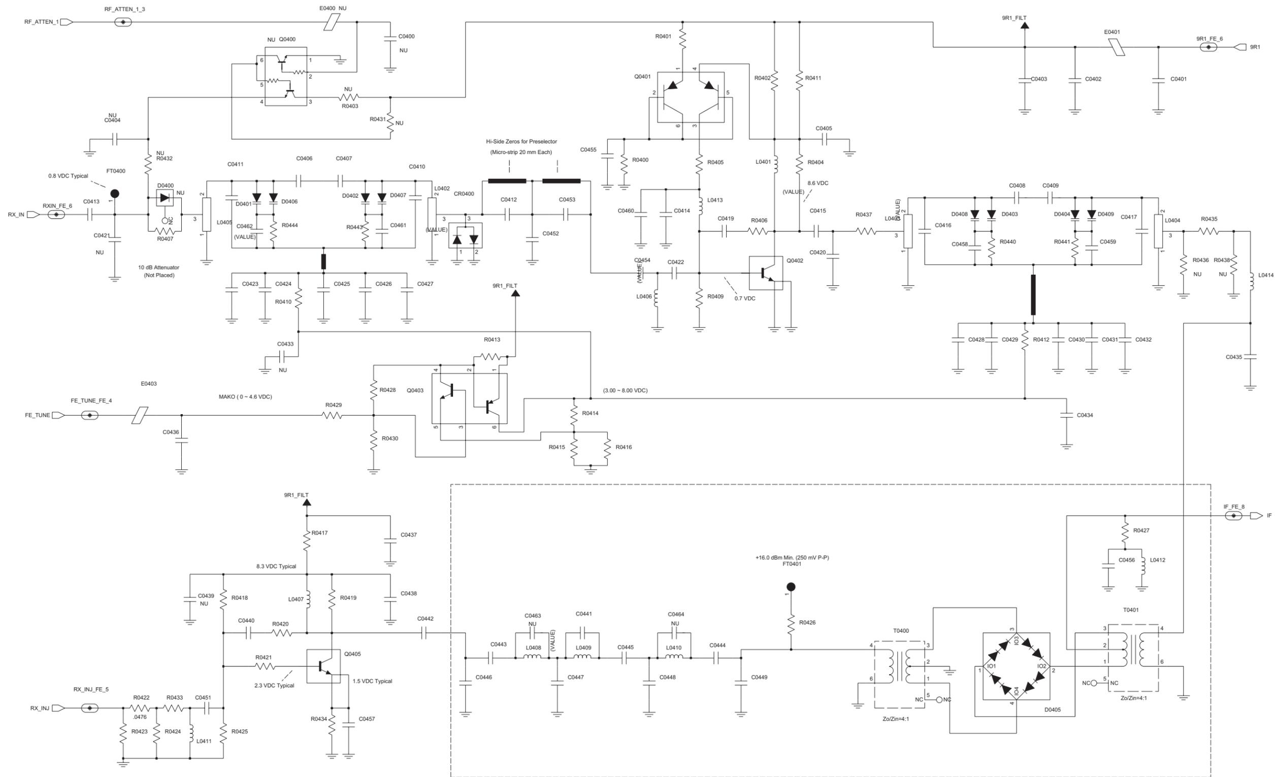
UHF2 (450–527 MHz) 1–40W Receiver Front-End Schematic Diagram
