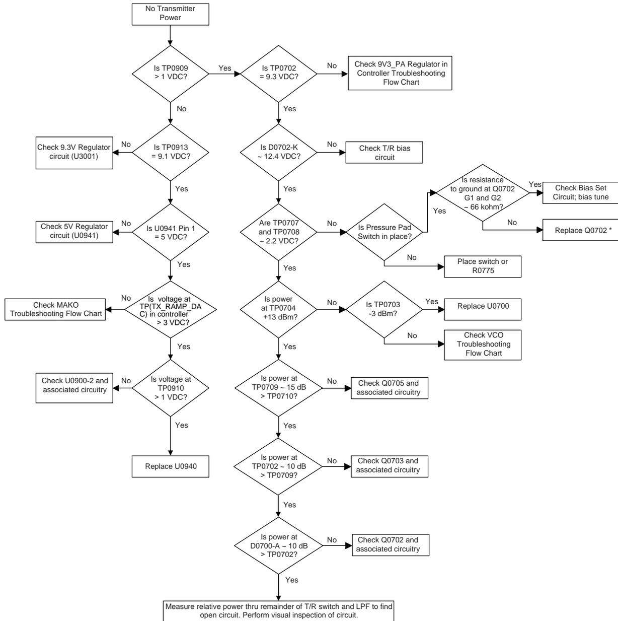
\* Note: If Q0702 is replaced, radio must be bias set and power set.
