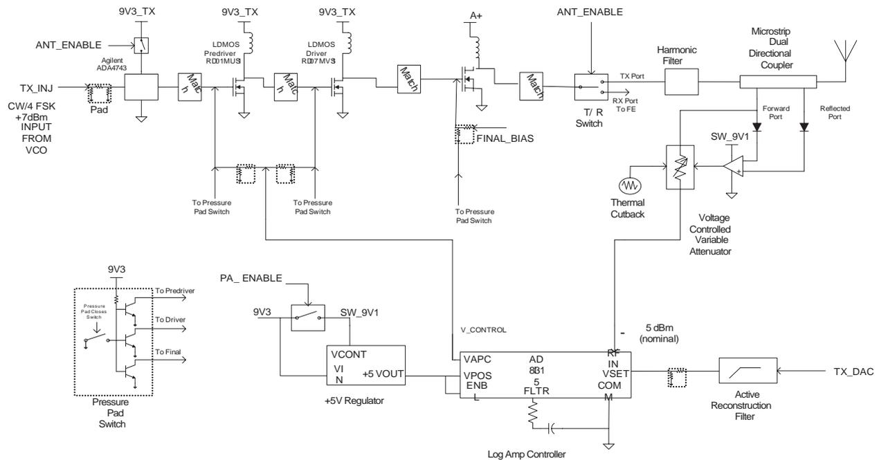
Figure 1-8 VHF 45 Watt High-Power Transmitter Detailed Block Diagram
