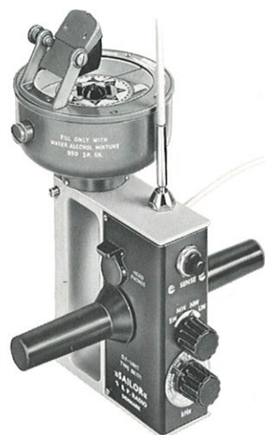
Ferrite Navigator BK171 For use in small plastic or wooden craft. This ferrite direction finder is equipped with a detachable 0.5-meter sense aerial. This feature, in conjunction with a 5-meter connecting cable and provisions for connect- ing headphones to the Ferrite Navigator makes operation outstandingly simple. Insensitive to heeling (sailing boats). The fixed-mounted bear- ing compass may also be used for optical com- pass direction finding. The Ferrite Navigator is not suitable for use in metal vessels.
