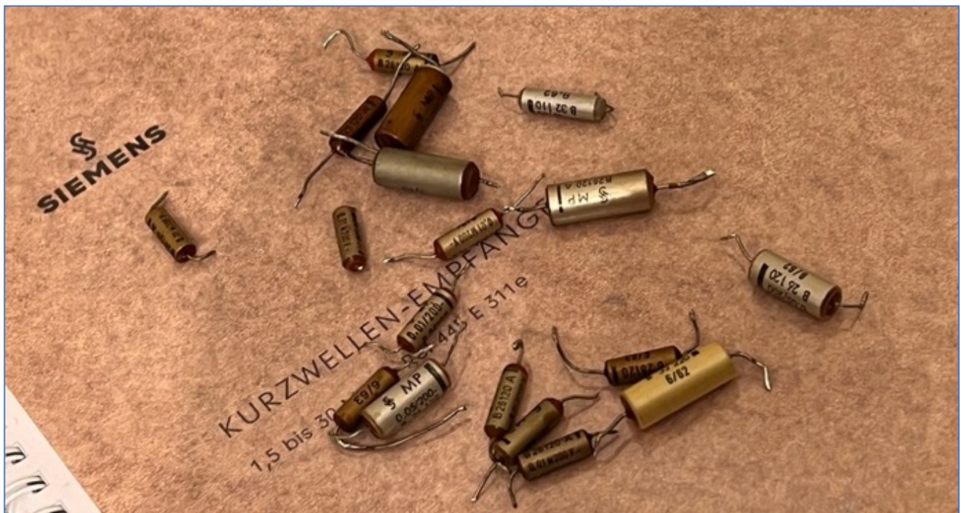
Some of the replaced MP capacitors
