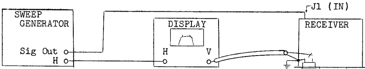
(2) Preliminary Adjustments. Disconnect the lead with violet insulation which is normally connected to the meter terminal and connect to the vertical deflection of the display unit (see test set up).
