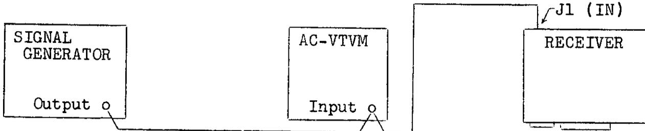
(2) Preliminary Adjustment. Set signal generator to 250 KC and an output level of .776 volts as indicated on the AC-VTVM. Set controls in the following table to the designated positions.
