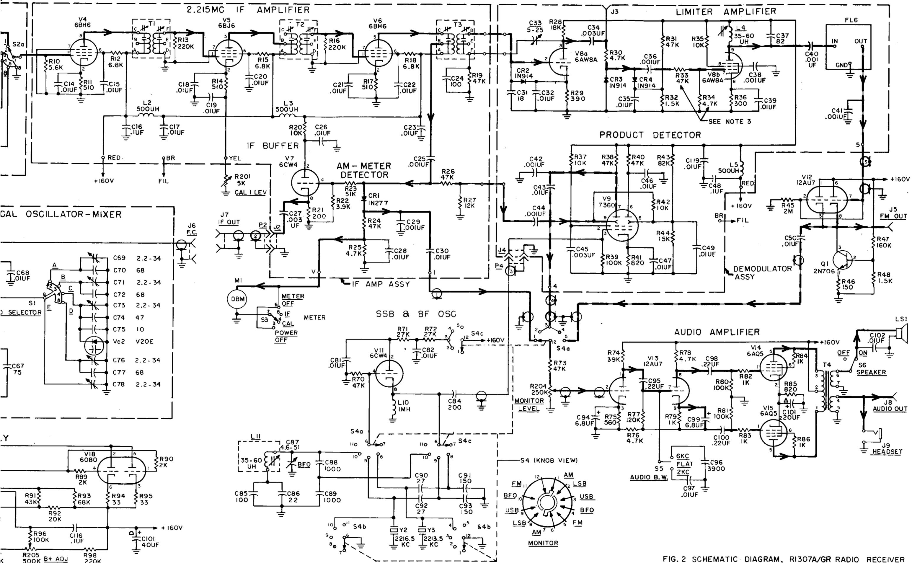
FIG. 2 SCHEMATIC DIAGRAM, RI307A/GR RADIO RECEIVER
