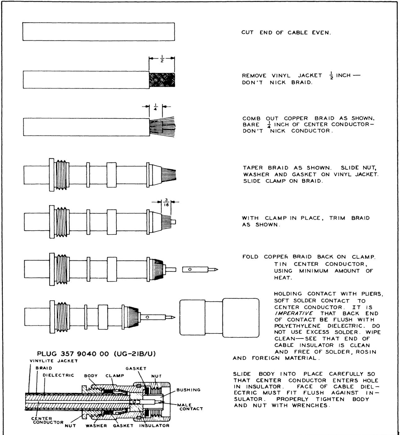
Figure 5-6. Assembling Plug UG-21B/U to Cable RG-8/U
