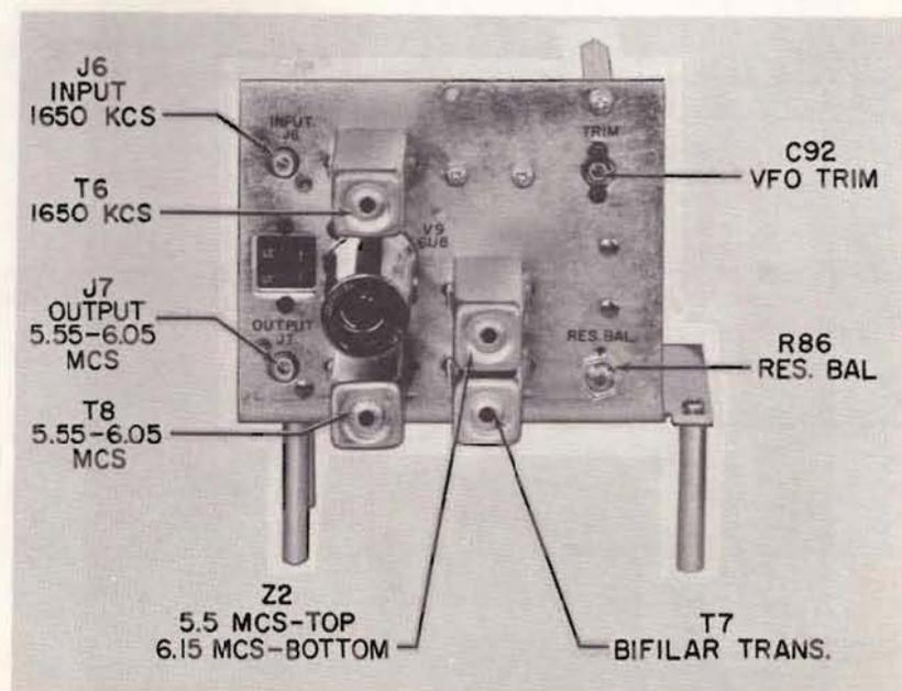
Figure 9. Top View of VFO Assembly Subchassis
