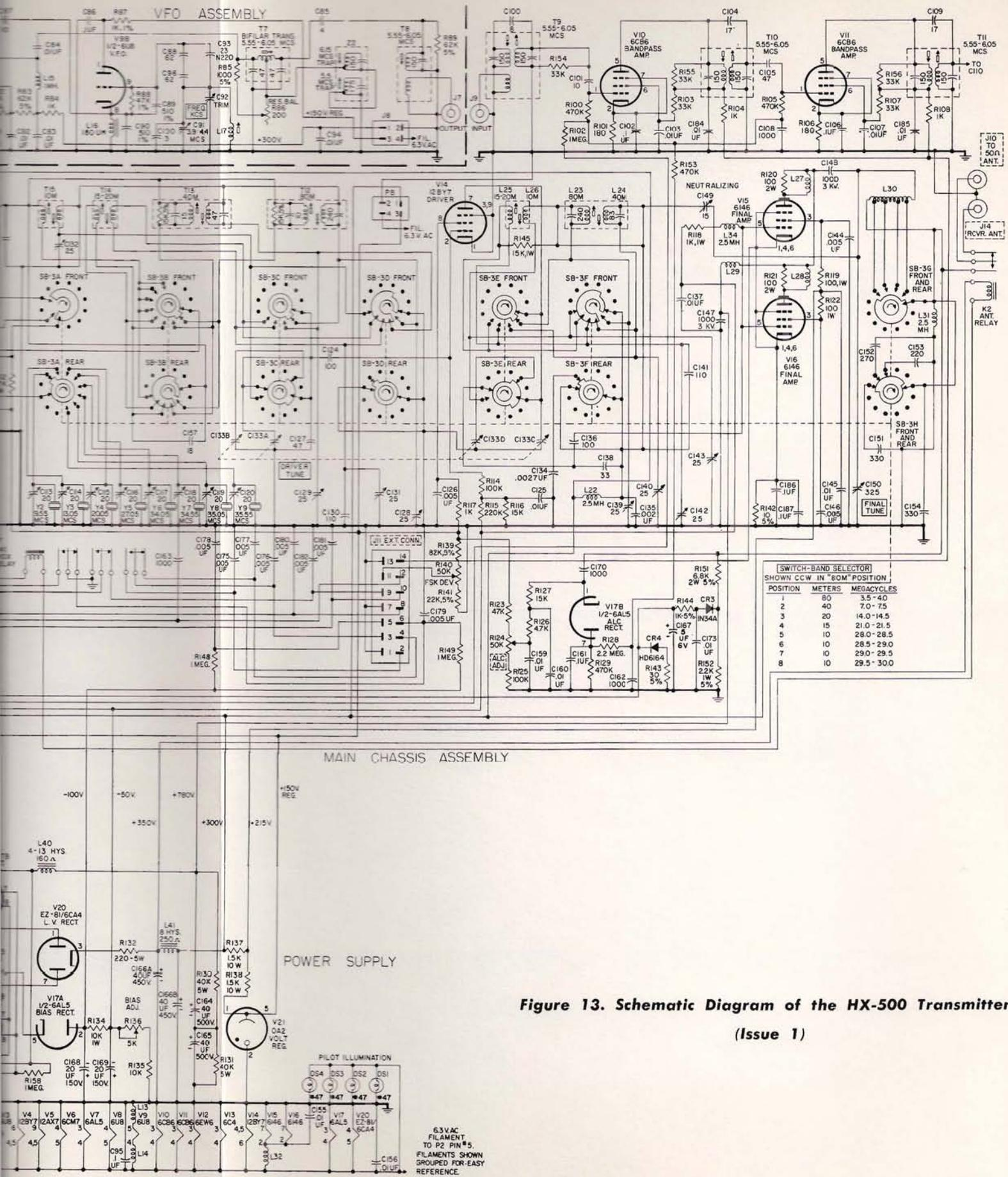
Figure 13. Schematic Diagram of the HX-500 Transmitter (Issue 1)
