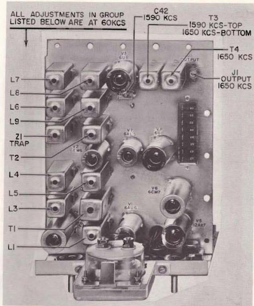
Figure 8. Top View of Exciter Assembly Subchassis
