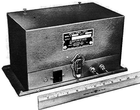
A vibrator power supply designed specifically for the T-90 Bandmaster Transmitter. Provides all necessary voltages. May be used with either 6 or 12 volts D.C. by changing jumpers. Comes complete with 10 foot shielded multiconductor output cable and connectors.
