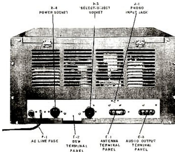
Figure No. 4. Rear View of Receiver
