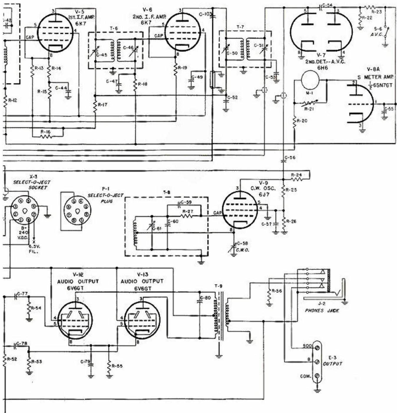
Figure No. 13. Schematic Diagram, HRO-50 Radio Receiver
