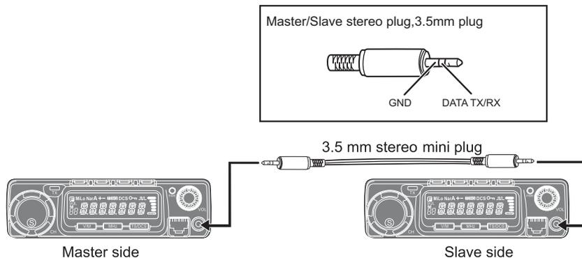
3. Press master unit's **[PTT]** key, LCD displays "SD XXX", "XXX" indicates data volume in transmitting. Slave unit displays "LD XXX", "XXX" indicates received data volume. When the transmission is successfully finished, the master and slave unit both display "**PASS**". Turn off the power, disconnect the cable and repeat step 2 to step 3 operations to clone the next slave unit.
