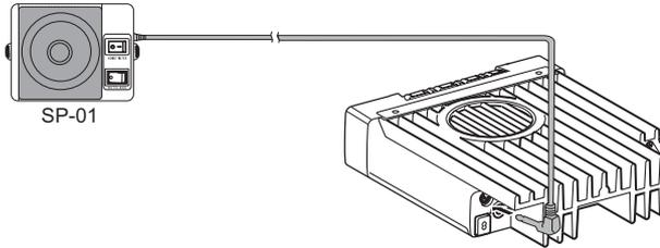
**NOTE** External speaker adopt double port BTL, please care about the connecting way. The speaker can not connect with the ground, otherwise the speaker will be fault. The wrong connecting way as the following picture.
