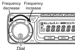
frequency in screen will be auto-hidden. In this status, turn selector knob or Microphone **[UP / DOWN]** key will increase or decrease frequency quickly by 1MHz step.
