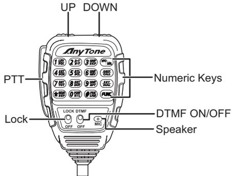
You can operate the transceiver by keypad or input desired frequency or channel through the QHM-03 microphone (Note:In professional transceiver mode,other keys are invalid except PTT,[ **UP** / **DOWN** ], **ONE CALL** and **SET DTMF** ).
