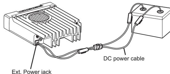
optional QCC-01(For Cigar-Plug connection) cable. Connect one of the cables between the ACC terminal or a Cigar-Plug that operates with the vehicle ignition or ACC switch on the vehicle and EXT POWER jack on the rear side of the unit.
