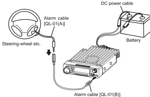
Connect DC power cable with car battery.
