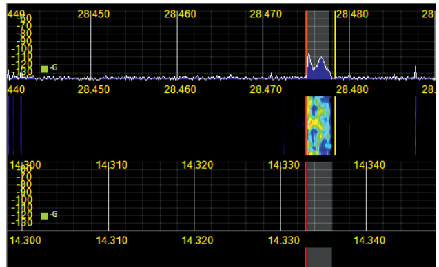
Figure 4 — A portion of the spectrum display in the panafall mode.
