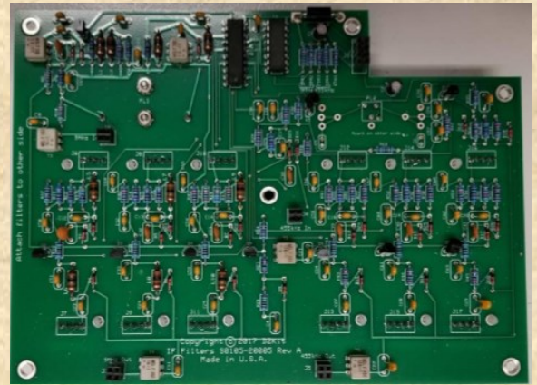
IF Filter board. Crystal filters plug in from the bottom
