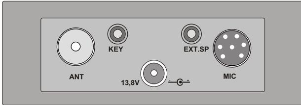
1. ANT - connect the HF/50MHz/70MHz antenna
