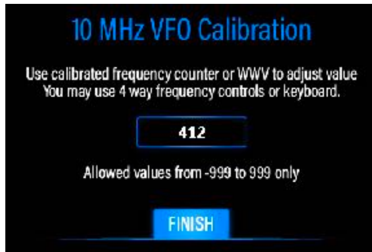
FIGURE 9: ADJUSTING VFO ACCURACY
