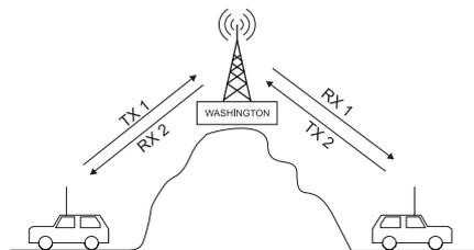
Once set up, your radio will automatically transmit the message received on the RX reception channel to the TX transmission channel. The duration of the message is limited to 5 minutes.
