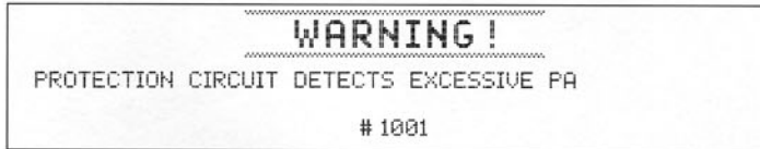
● Typical Protection Alert Display
