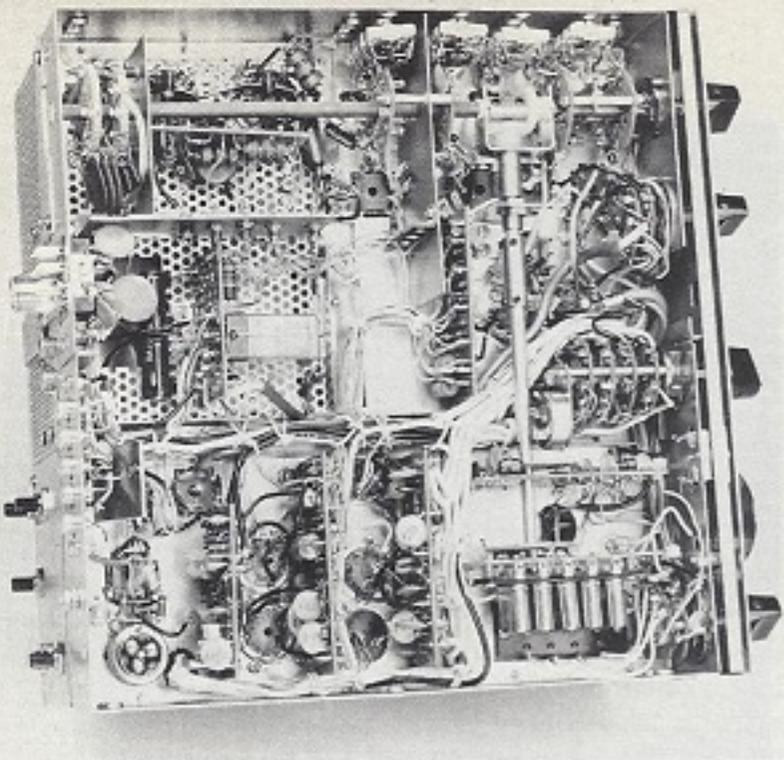
Bottom view of the T-4XC. In this picture the final amplifier is at the top left, with the driver stage at the top right.
