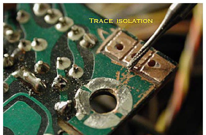
Figure 7 - Scrape away the copper between each hole to make a solder pad for each leg/terminal of the 7808.
