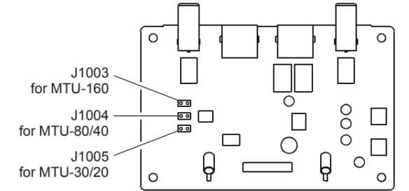
For example, if your μ-TUNE-UNIT is MTU-80/40, insert the Jumper Plug to the J1004 that is labeled MTU-80/40.
