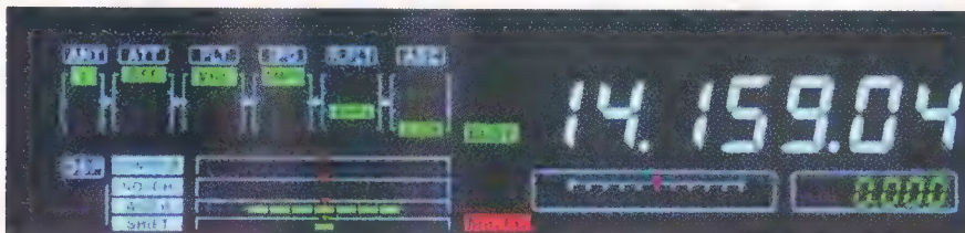
Photo 2 - The main receiver part of the bright, multi-coloured main display which includes a “block diagram” of the receiver front end, showing the antenna, attenuator, pre-selector, pre-amp, roofing filter and AGC settings in use.
