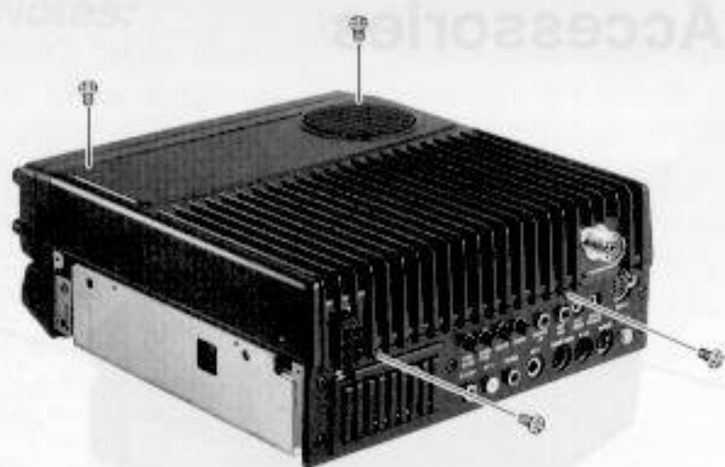
Fig. 4: Top Cover/Heatsink Removal
