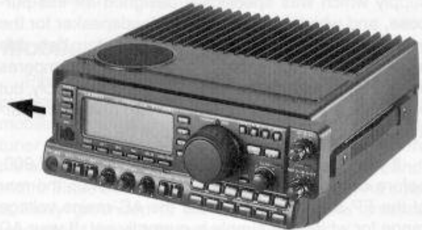
Installing the Front Sub-Panel
