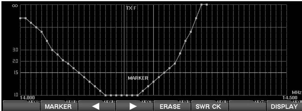
1. Press the [2/3.5](**MARKER**) key to turn the marker function on; the marker cursor will be displayed.
