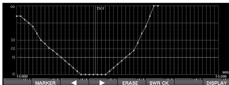
In order to measure the SWR of the antenna system correctly, please turn off the antenna tuner before measuring the SWR.
