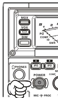
**Note:** The opening screen will appear on the after-market monitor to the DISPLAY, and the self-check function of the CPU inside the radio will begin. Then, the  $\mu$ -Tuning circuitry will receive the data from the CPU, and it will perform its own self-check, and will preset itself to the proper settings for the current operating frequency.
